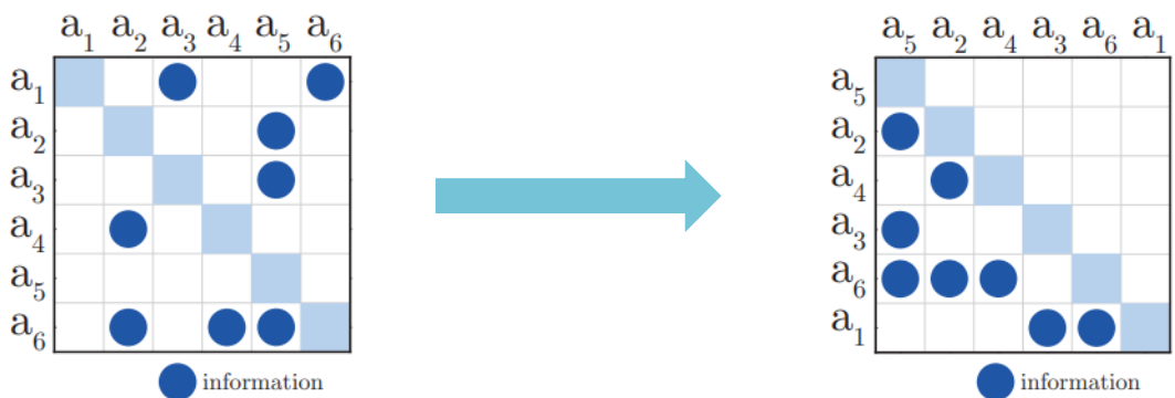
Figure 4: Illustration of a sequenced process DSM (from (Wilschut 2018)).
