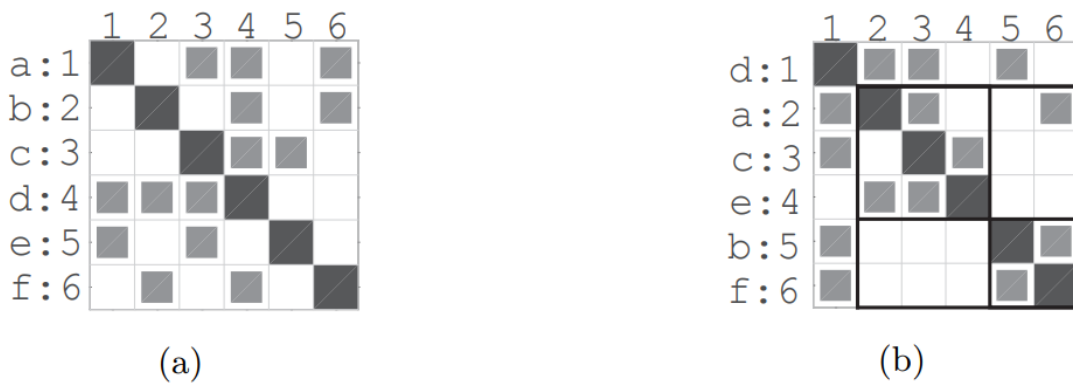
Figure 3: a) Unclustered example of a DSM and b) clustered DSM (from (Wilschut 2018)).
