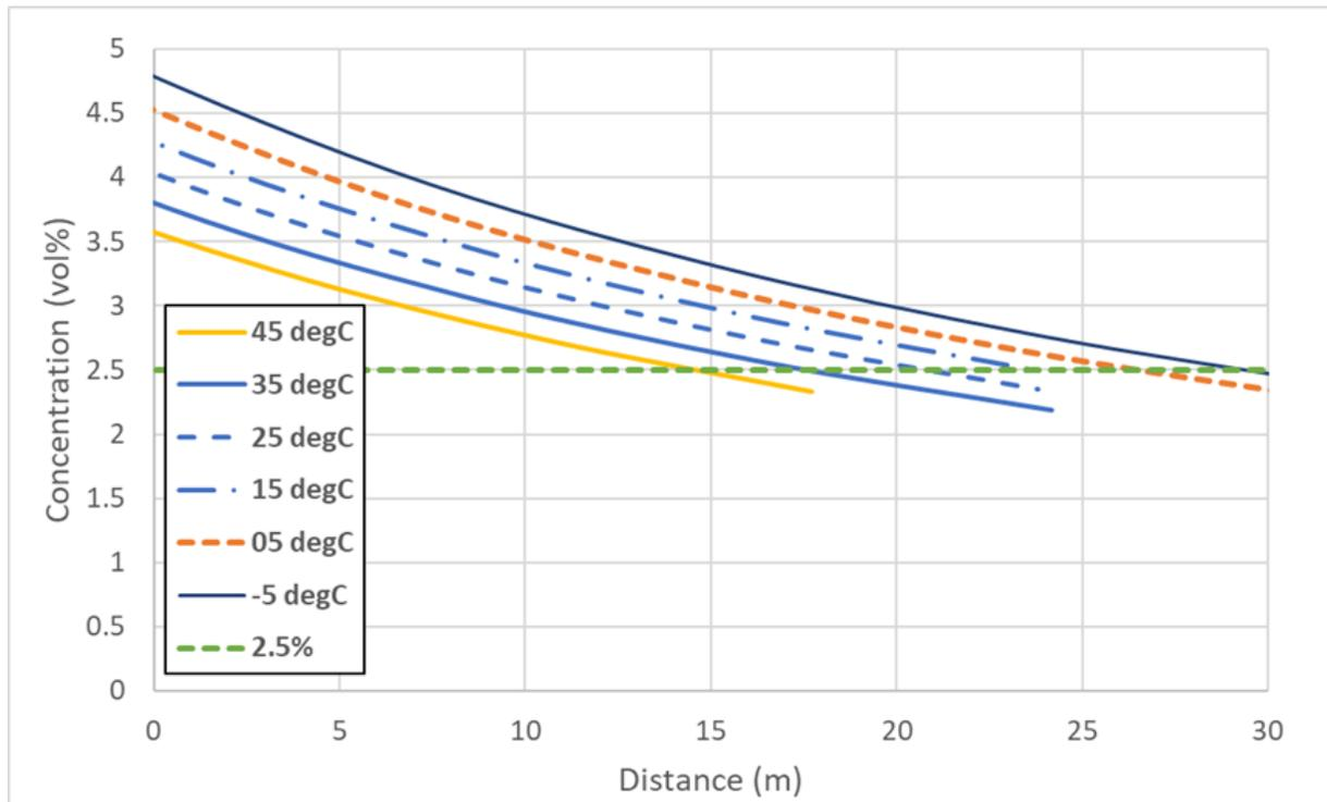
Figure 5.12 Concentration vs distance for changing outflow temperatures.
