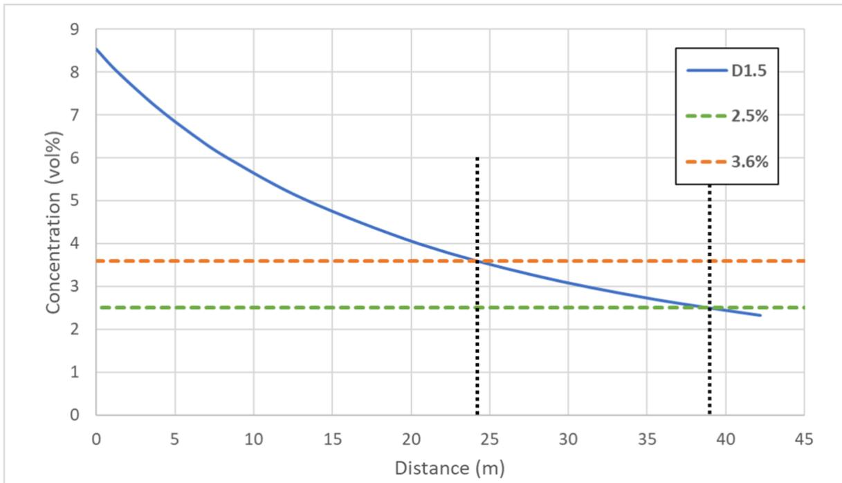
Figure 5.5 Concentration oxygen as function of distance. The orange and green horizontal lines represent 3.6 vol% and 2.5 vol% oxygen, respectively.
