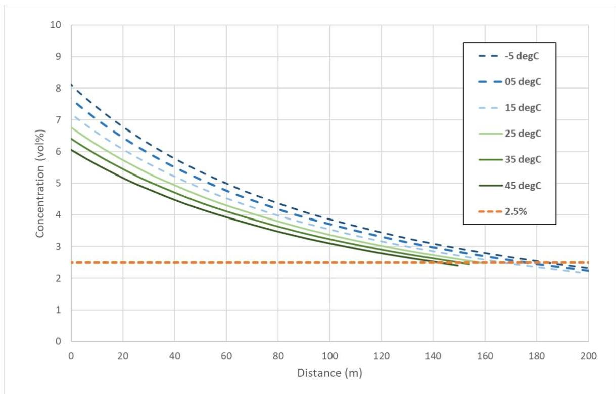
Figure 5.14 Concentration as a function of downwind distance.
