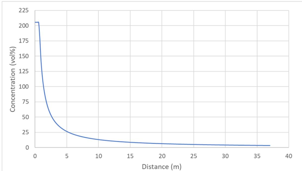
Figure 5.4 Concentration vs vertical distance to release point in oxygen jet.
