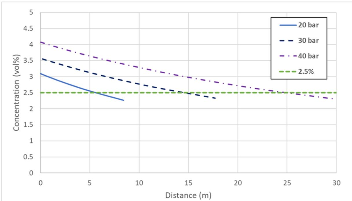
Figure 5.11 Concentration vs distance for varying PEM operating pressure.
