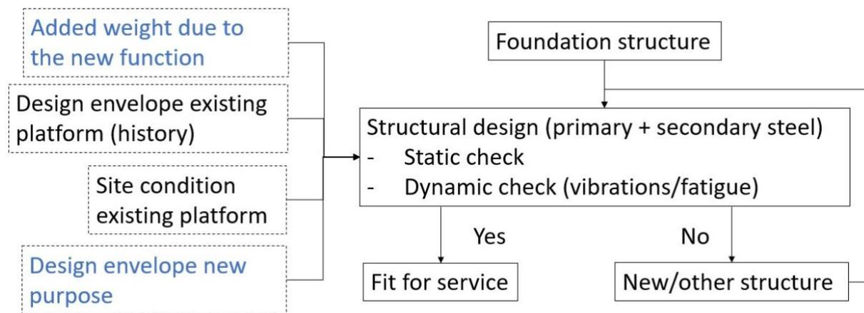
Figure 3.1: Visual for re-assessment of structural integrity of foundation structure for re-use
