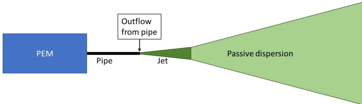
Figure 5.3 Schematic representation of used models for oxygen dispersion.
