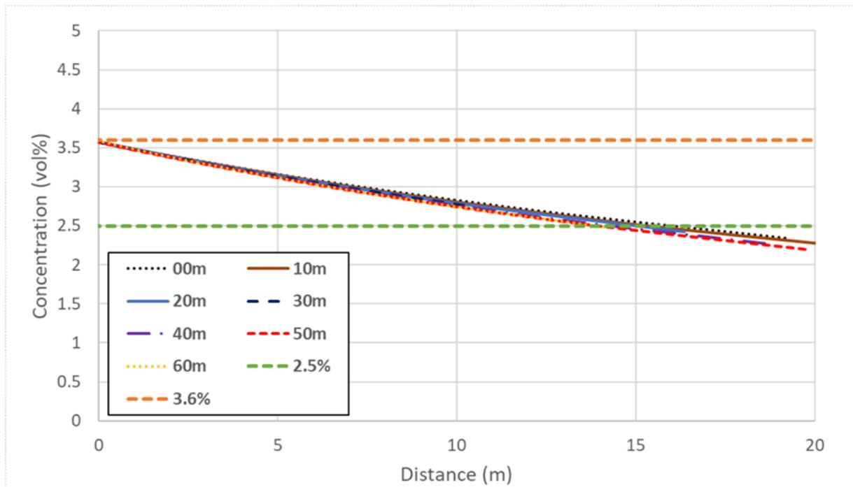
Figure 5.9 Concentration vs distance for varying release height.
