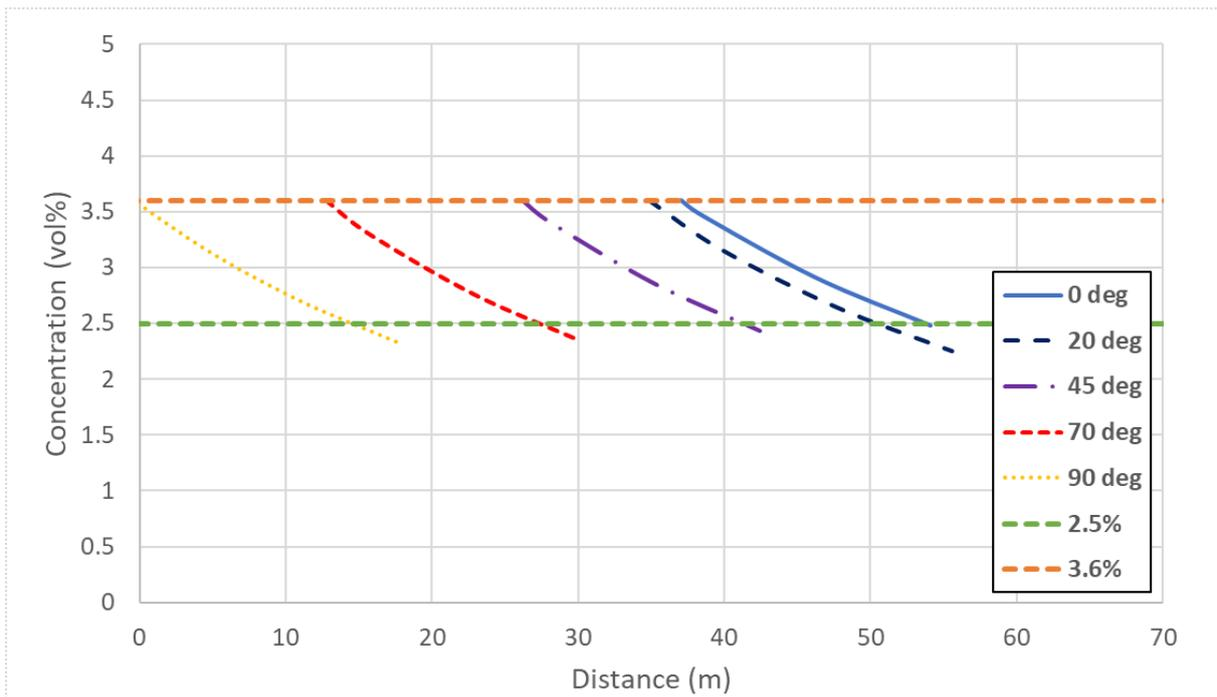
Figure 5.8 Concentration in dispersion model versus horizontal distance for various outflow directions ; horizontal: (0°) to vertical (90°). Lines start at horizontal distance of end point jet model.
