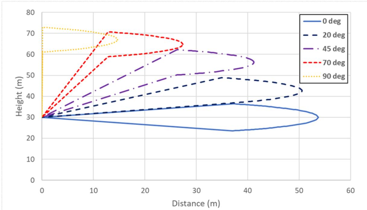
Figure 5.7 Cloud side view for various outflow directions.
