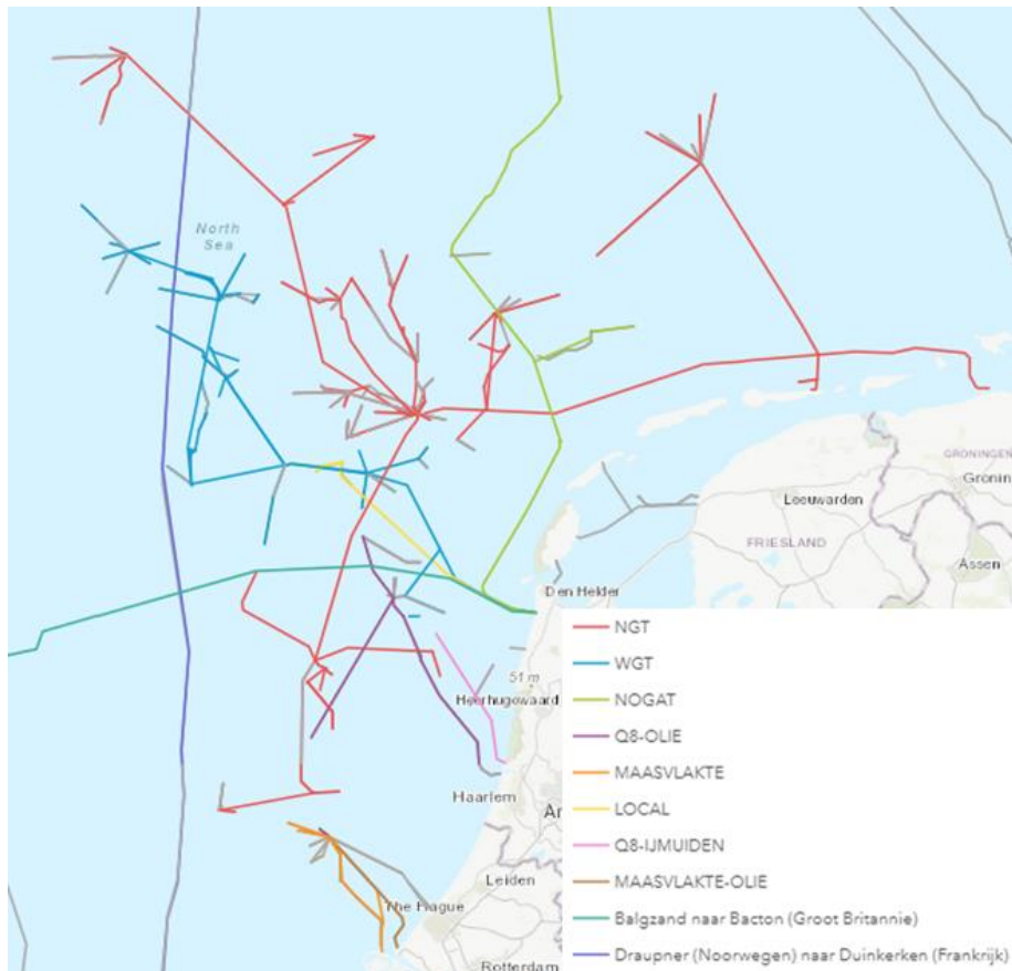
Figure 4 Natural gas pipelines on the Netherlands Continental Shelf
