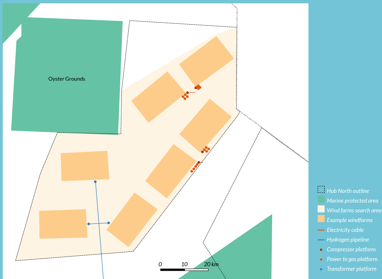
Figure 6. Map of the standard design of Hub-North. Note that the exact placement of example wind farms, platforms, and pipelines and cables is illustrative and not used in the impact assessment.
